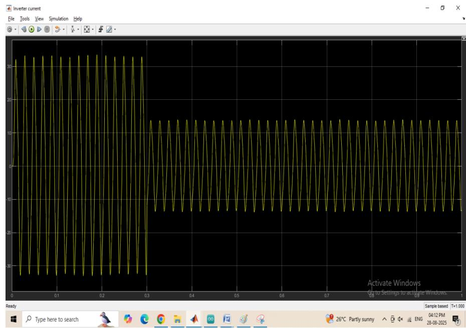
The inverter current is around 32A. The efficiency of the proposed inverter is provided below:
