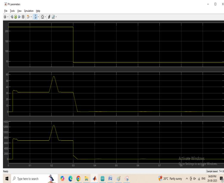
The PV converter operates at approximately 240 V with a current of 30 A, delivering a power output of approximately 7100 W. The grid voltage and inverter output voltage are depicted in the following figure:
