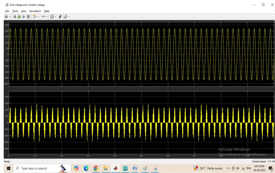
The inverter output voltage is approximately 240 V, while the grid voltage is around 220 V. The load power is illustrated in the following figure:
