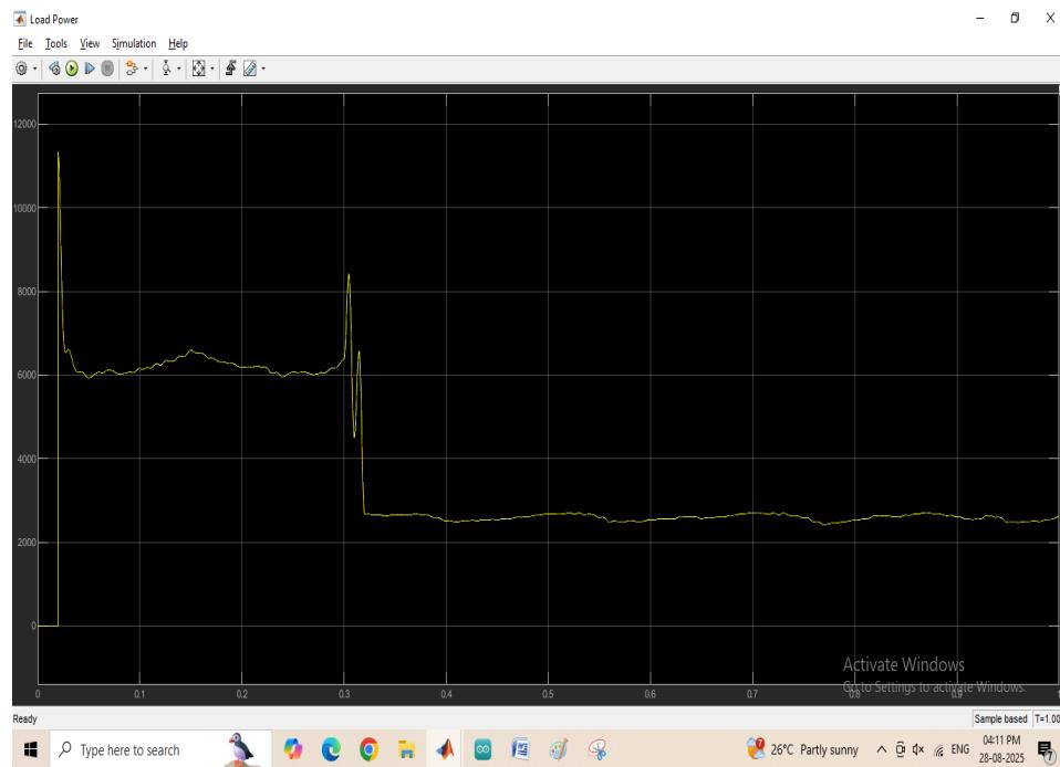
The load power is around 6600W. The load current is provided below:
