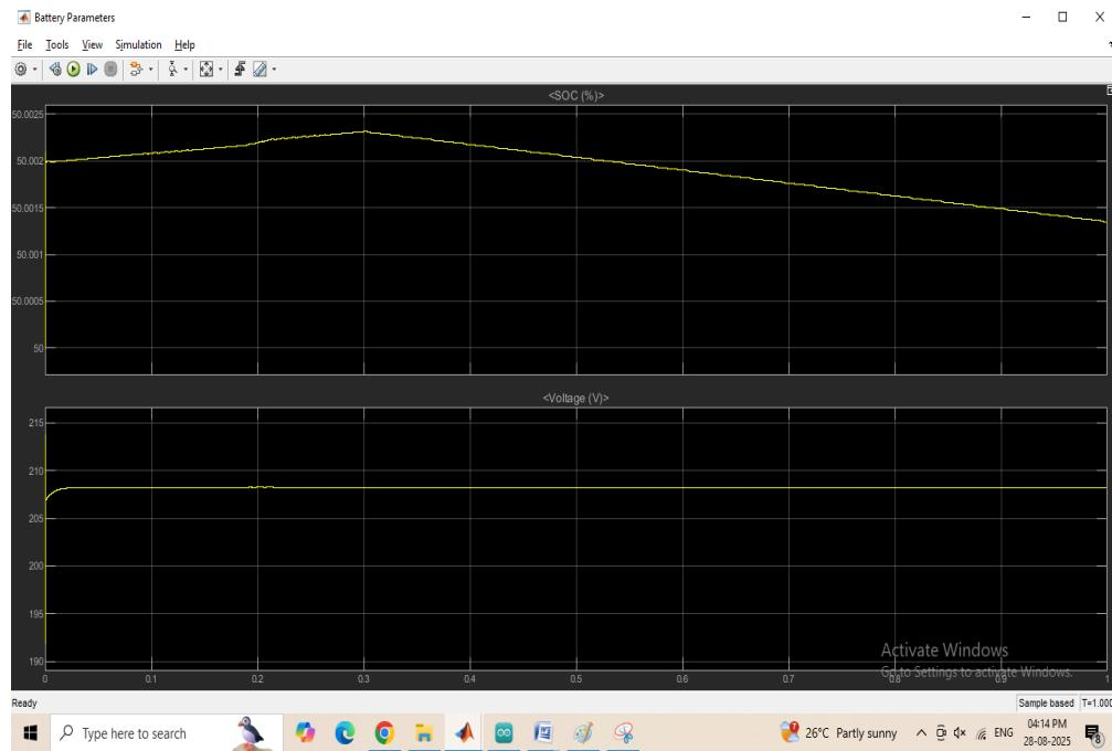
In this the battery is charging until  $t=0.3s$  when PV source is available and %SOC is increasing and when PV is not available, battery is discharging and SOC is reducing.
