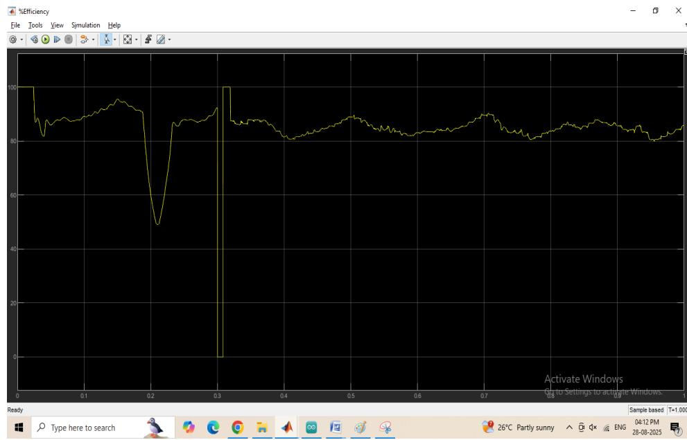
The efficiency is around 88%. The battery %SOC and voltage is provided below:
