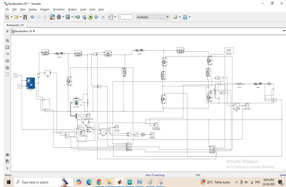
In this configuration, a PV source rated at 105 V and 7200 W supplies power to the inverter, which steps up the voltage to 230 V for injection into the grid. A battery with a voltage of 192 V and a capacity of 4.5 Ah serves as a secondary power source. The PV voltage, current, and power characteristics are presented below:
